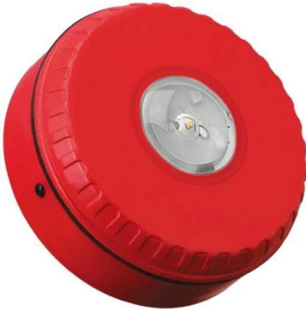
The Solista LX Ceiling has a unique lens design that distributes the light in a cylindrical shape to achieve the required illumination specified by AS ISO7240.23:2014. Designed for installation at a height of up to 3m and with a discrete appearance, the device is ideal for a variety of applications, including bedrooms, bathrooms and toilets.
